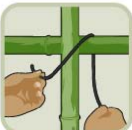
Weave around the joint.
