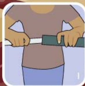
1 Sheath the pipe with foam.
