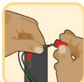
Insert the wires into wire nuts.
