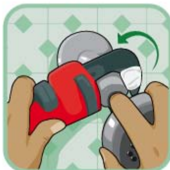
Loosen the showerhead from the pipe.
