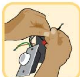
Twist matching wires together.
