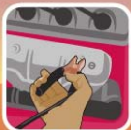
Ground to the engine block.
