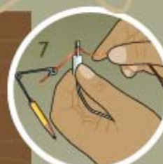
Wrap the wire around the safety pin and the earphone's receptor.
