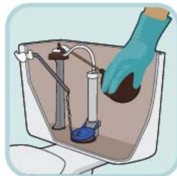
Check the flush ball for leaks.
