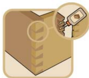
Cut the tail board joint.
