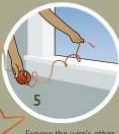
Expose the wire's other end—it acts as an antenna.
