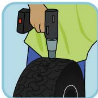
Drill three holes for drainage.
