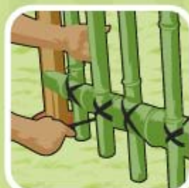
Tie each juncture.
