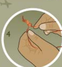
To lengthen your wire, twist on a second one.
