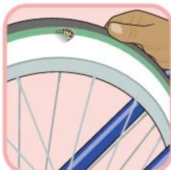
Find the hole; pull the tire off the rim.
