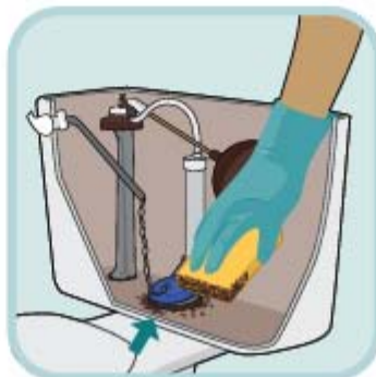
Clean the flush valve seat.
