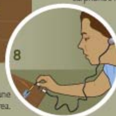
Wrap the wire around the safety pin and the earphone's receptor.
