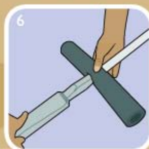
6 Slide onto the bare pipe end.
