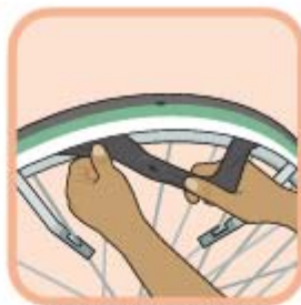
Pull out the damaged tube.
