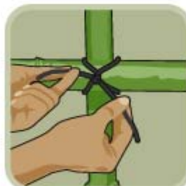
Knot behind the joint; trim.
