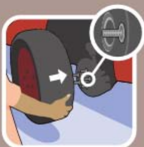
Put a spare over the studs.
